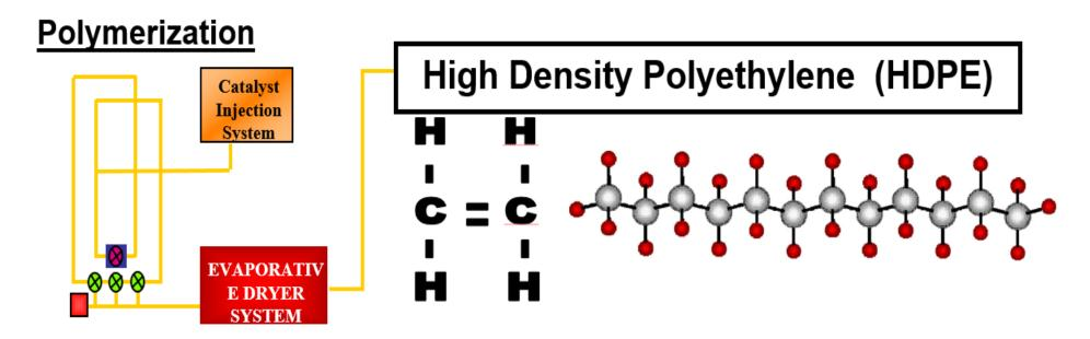
HDPE resin is derived from simple hydrocarbon polymer chains where the Ethylene molecules form a simple repeat structure (basically two carbon atoms and four hydrogen atoms repeated over and over again). From a molecular standpoint nothing is gained and nothing is lost.
