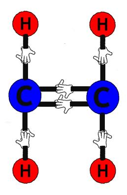
Ethylene is a gas that is extracted from a hydrocarbon source such as crude oil or natural gas and its basic molecular structure is formed by 2 Carbon atoms holding on to each other with two hands (double bond), and each of the remaining hands holding onto a Hydrogen atom (single bond). This is the basic building block (monomer) for many well known polymers we know as plastics.
