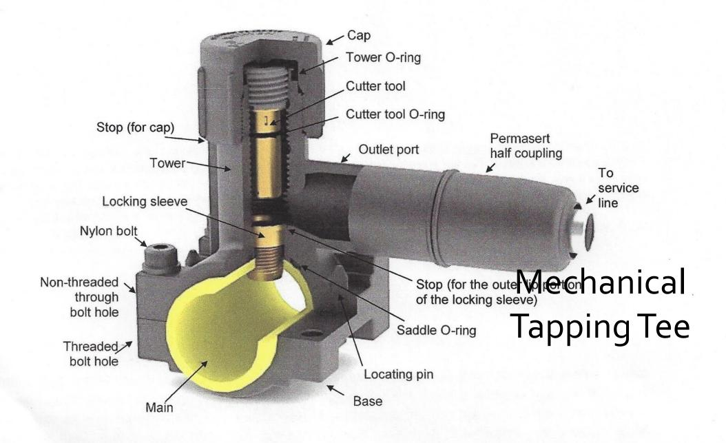
Figure. Cross-section diagram of an exemplar PermaLock mechanical tapping tee assembly,
